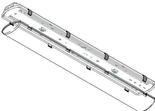
7. SECURE DIFFUSER/LENS WITH CLIPS
