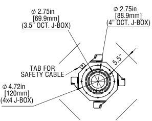
HINT: For ease of engaging the fixture to the mounting bracket, it is recommended to draw temporary lines parallel to the straight edges of the bracket (as shown above), use those line to line up your fixture before you twist and lock the fixture onto the bracket.
