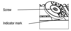
Loosen the screw to adjust the angle. Retighten once the angle is set.
