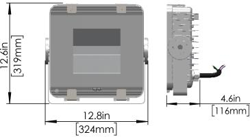
1. Install the fixture to designated location, and use dimension below for bolt's location.
