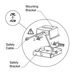
3. Install the fixture by snapping mounting bracket into safety bracket.
